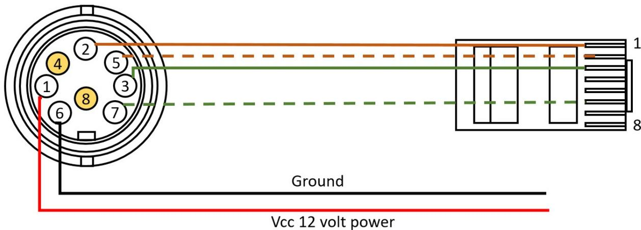
*This is the front view; holding the connector by the wires and viewing the terminals.*
