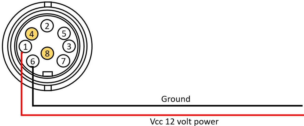
*This is the front view; holding the connector by the wires and viewing the terminals.*
